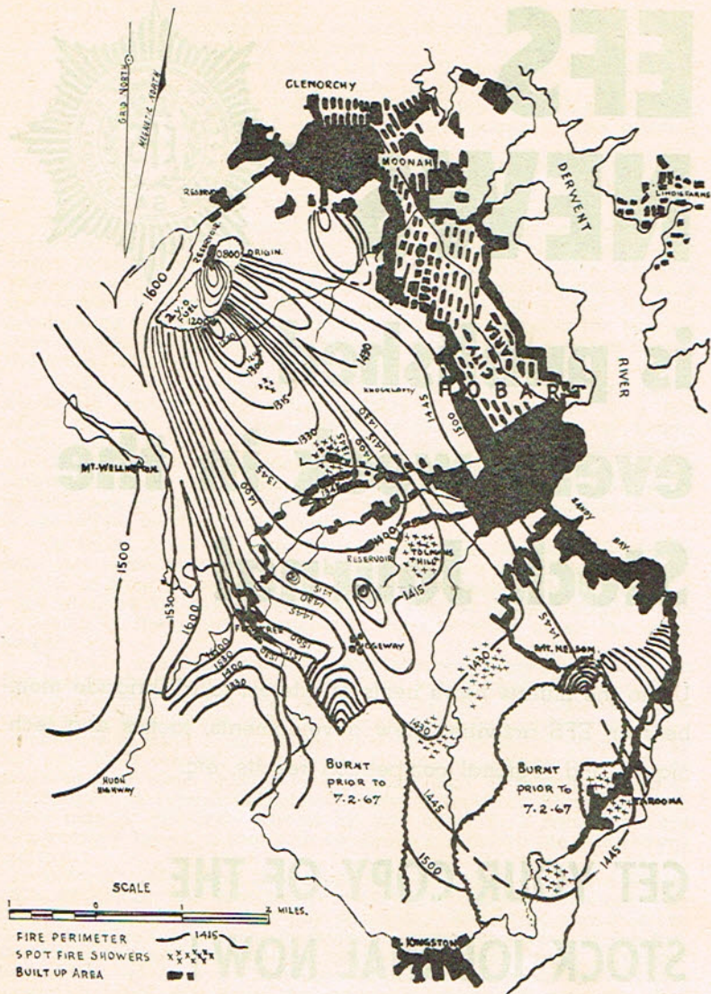
FIGURE 2—Plan showing origin and progress of the Hobart fire on February 7, 1967. The location of the main areas of spot fire showers which caused the tremendous acceleration effect are shown in relation to the headfire travel.
